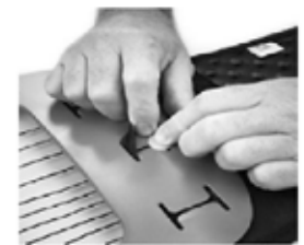
4. Slide rivet head to end of slot to remove
